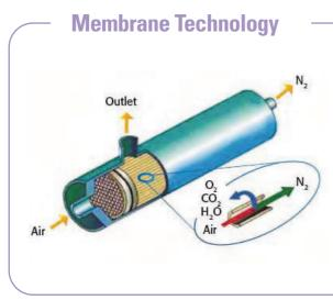
Compressed air is forced through a hollow fiber membrane, with selective permeation of the different components - nitrogen, oxygen, CO<sub>2</sub>, water vapor and traces of rare gases - depending on the rate of diffusion. The rate of diffusion of nitrogen trough the membrane is slower than the other components, which thus flow outside of the fiber membrane, leaving just nitrogen inside; this is then discharged subsequently,
